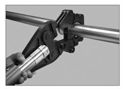
8c. After the pressing operation is complete, release the Vic-Press adapter jaw from the Vic-Press ring by squeezing the levers. Remove the tool from the Vic-Press ring.
