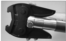
7. Install the standard Vic-Press jaw or Vic-Press adapter jaw into the tool. Make sure the standard Vic-Press jaw or Vic-Press adapter jaw aligns properly to permit insertion of the locking pin.
