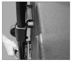
1. Engage the upper bracket of the dolly with the upper bar on the back of the tool or accessory case, as shown above.
