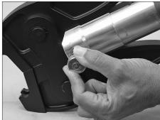
7a. Push the locking pin fully into the tool until it clicks.
