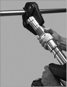
5. Place hands, as shown above. Keep hands away from the standard Vic-Press jaw and other pinch points at all times during the pressing operation. **NOTE:** The cylinder of the tool can be rotated for ease of alignment.
