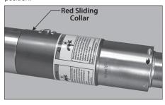
The position shown above (red sliding collar engaged in the upper/forward position) must be used for ½-inch/21.3-mm and ¾-inch/26.9-mm sizes.
