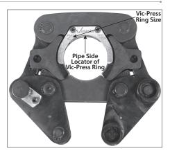
2. Select the proper size Vic-Press ring for the fitting and pipe size being installed. **NOTE:** The Vic-Press ring size is stamped on the "pipe side" locator of the Vic-Press ring.
