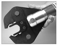
2. Open the standard Vic-Press jaw by squeezing the levers.
