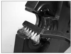
5. Remove deposits from the pressing cavities of the standard Vic-Press jaws with a wire brush.
