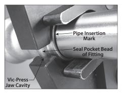
4. While positioning the standard Vic-Press jaw, make sure the pipe remains inserted fully in the fitting and that the Vic-Press jaw cavity aligns/ engages with the seal pocket bead of the fitting, as shown above. The end of the fitting must be flush with the pipe insertion mark. Always refer to the I-P500 Field Installation Handbook for pipe preparation and marking requirements.
