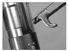
2. Clean the drive rollers and the locking pin with a brush or compressed air.
