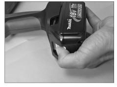
1. Remove the battery from the tool by depressing the button, as shown above.
