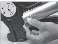
1. Release the locking pin by pushing in and turning counterclockwise. Use caution when releasing the locking pin. The locking pin is under spring-loaded pressure. Remove the standard Vic-Press jaw or Vic-Press adapter jaw from the tool
