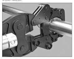
7. Engage the Vic-Press adapter jaw hooks into the Vic-Press ring, and release the levers. Make sure all four hooks of the Vic-Press adapter jaw engage completely with the Vic-Press ring. 7a. While positioning the standard Vic-Press adapter jaw and Vic-Press ring, make sure the pipe remains inserted fully in the fitting. The end of the fitting must be flush with the pipe mark. Always refer to the I-P500 Field Installation Handbook for pipe preparation and marking requirements.
