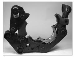
3. Pull the latching pin of the Vic-Press ring out until it disengages the Vic-Press ring arm. Allow the Vic-Press ring to open completely, as shown above.
