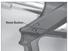
2. Installation of the standard Vic-Press jaw or Vic-Press adapter jaw is possible only when the drive rollers are retracted sufficiently. If necessary, press the reset button until the drive rollers are retracted.
