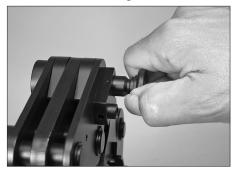
8d. Remove the Vic-Press ring from the fitting by pulling the latching pin out until it disengages the Vic-Press ring arm, as shown in Step 3 of this section.
