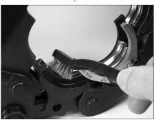
6. Remove deposits from the pressing cavities of the Vic-Press rings with a wire brush.
