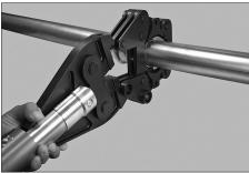
6. Install the Vic-Press adapter jaw into the tool by following the "Tool Setup" section.
