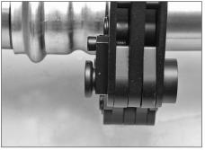
5. Close the Vic-Press ring by aligning the holes of the two ends. Push the latching pin through the Vic-Press ring arm completely, as shown above. **NOTE:** The Vic-Press ring can be rotated around the fitting for ease of tool positioning.
