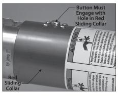
6. After adjusting the red sliding collar to the appropriate position, make sure the button is engaged completely with the hole in the sliding collar, as shown above. **NOTE:** The button will pop up with an audible click, ensuring that the red sliding collar is in the locked position.
